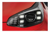
Day Time Running Lamp These LED lights keep running whenever the engine is on and increase the visibility of your cars for other vehicles on the
