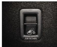
Child Anchor Keep your child safely and securely seated by strapping their seat to the vehicle using straps from the child safety seat that connect to special metal anchors in the vehicle.
