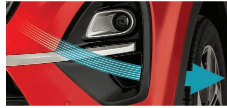
Aerodynamic improvements The smart rear-spoiler side garnish minimizes the drag coefficient for improved fuel efficiency while a state-of-the-art wheel air curtain improves the flow of air around the front wheels to offer you a more comfortable driving experience.
